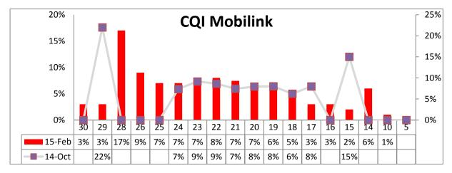
The CQI for Mobilink has improved and shows higher CQI assignment over the route as seen from the bar chart when compared with line chart. Similarly for Mobilink the CQI distribution is almost the same but comparatively have less contribution from good CQI values.
