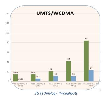
that enables them to implement Rel-7 (HSPA) of UMTS Technology. Under ideal conditions it can achieve a peak data rate of 21 Mbps (64 QAM) for downlink and 11 Mbps (16 QAM) for Uplink.
